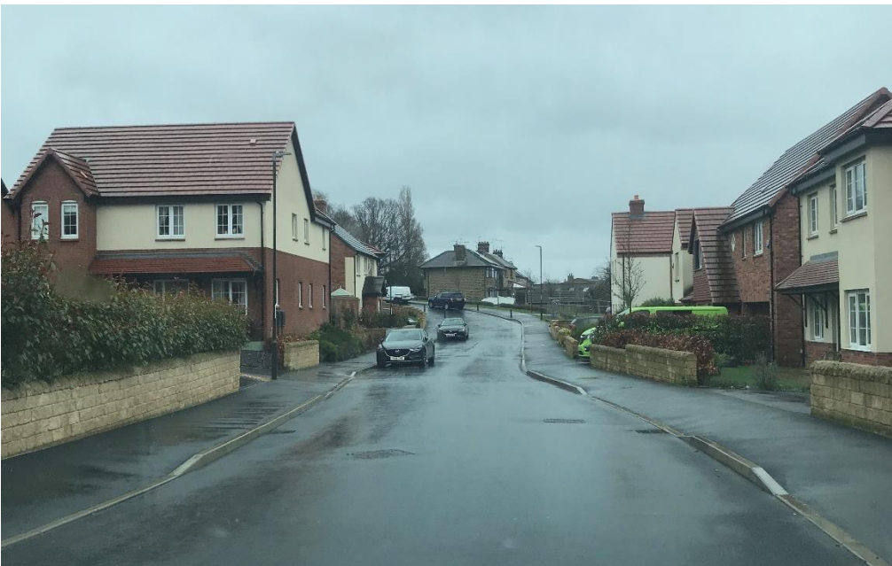
Figure AM-A5: On-street parking occurring on carriageway width of 5.5 metres
